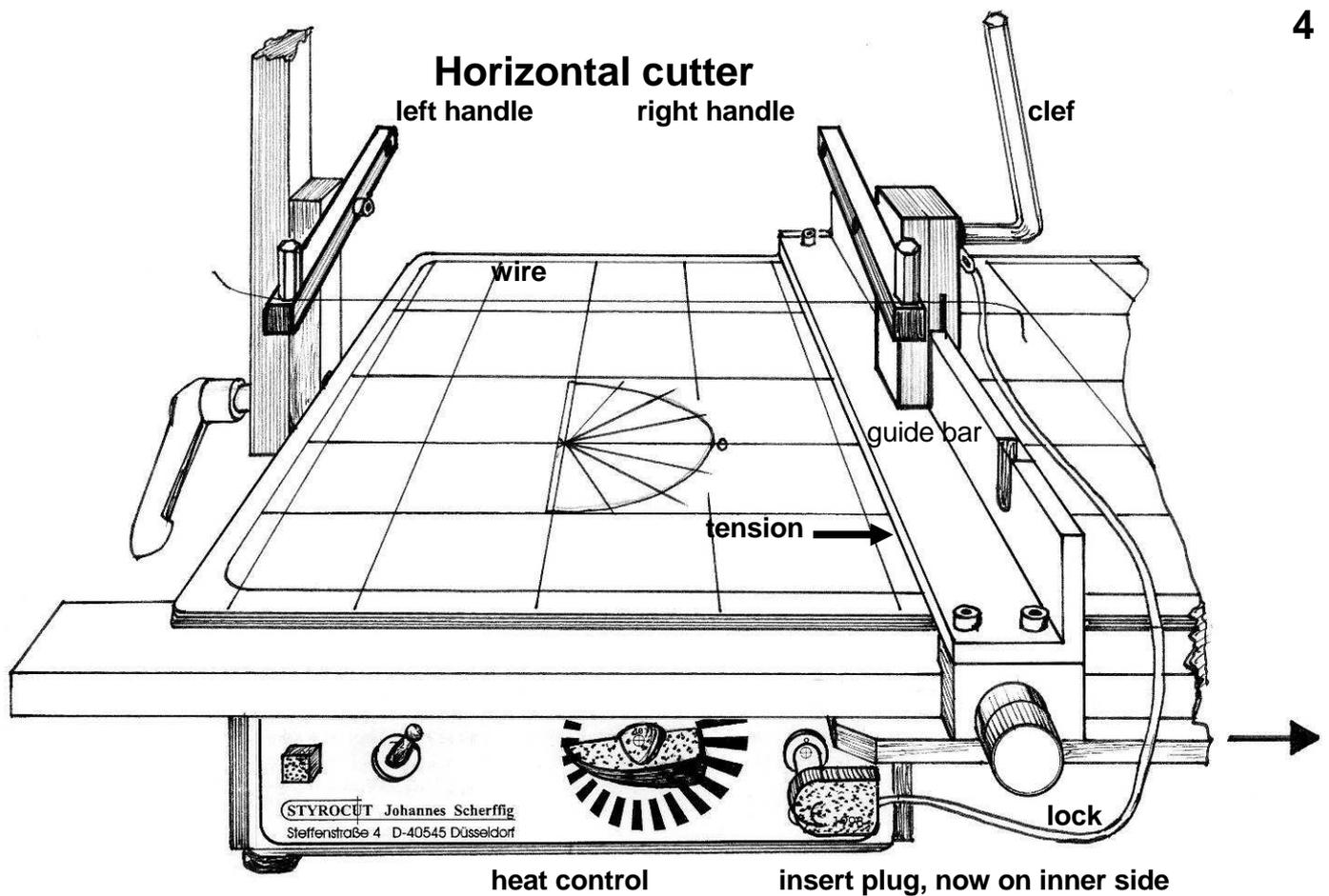
To set the cutting height, shorten a left-over piece of Styrofoam and lower the tight wire onto it. Cutting heights of less than 10 mm require a slice of at least 10 mm thick to be placed underneath and pushed through together. Cutting heights of more than app. 80 mm should be done with the second hole or thread in the handles.
